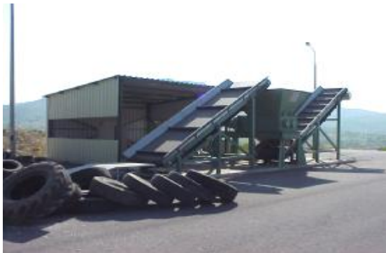
Figure 7: Shredder of useless tires
